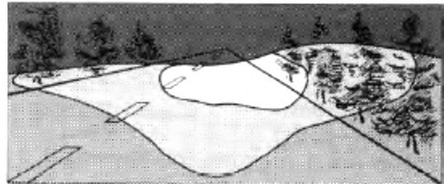
Light distribution with improved foreground illumination
